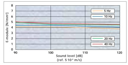
Amplitude relationship of the dynamic rigidity of Sylomer<sup>®</sup> S 600 in the usual excitation range for structural applications. Samples: 280 mm x 280 mm x 50 mm
